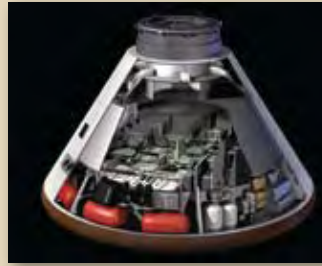
Figure 3 The Orion crew exploration vehicle will transport a new generation of explorers to the moon, with crewed flights scheduled to begin in 2015. This artist's rendering represents a cut-away concept of the Orion crew exploration vehicle's crew module.
