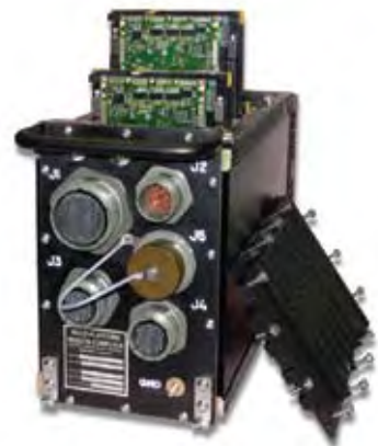
One of Curtiss-Wright's innovative family of PCOTS subsystems, the MPMC 350p houses up to 3 rugged DCP-124 PowerPC SBCs, Ethernet, Serial and DIO interfaces.
